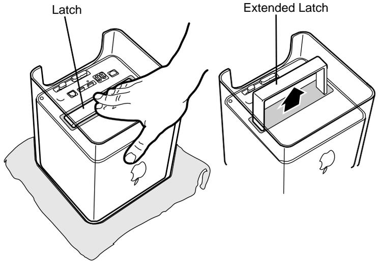
Allow the latch to extend completely.
