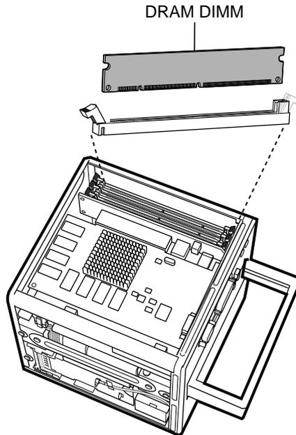
Your computer uses synchronous DRAM (SDRAM) DIMMs that must be compatible with the computer's specifications. Replace the DIMM in your computer with the replacement DIMM provided in this package. Do not use DRAM DIMMs from older computers, even if they fit into the DIMM slots.
