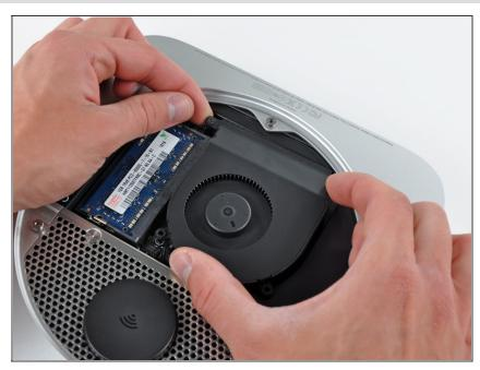
Lift the ear of the fan nearest the RAM up off the standoff secured to the outer case.
