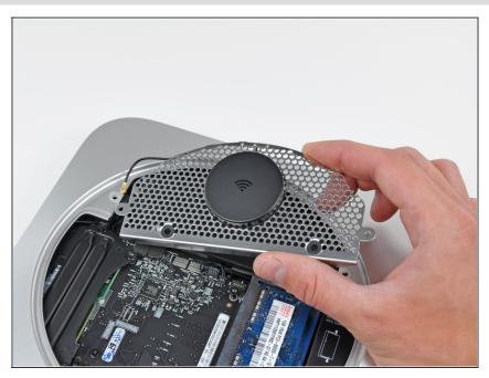
Remove the antenna plate from the mini.
