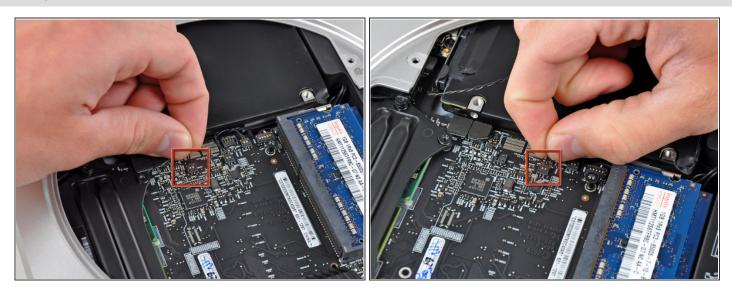
• Carefully pull the wires for both hard drive thermal sensors upward to lift their connectors up and out of their respective sockets on the logic board.
