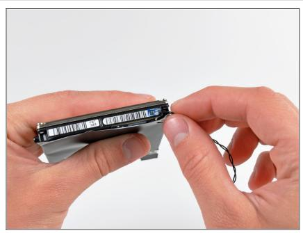
Carefully peel the thermal sensor off the end of the hard drive.
