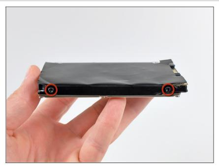
Remove the two 6.2 mm T8 Torx screws from the side of the hard drive.
