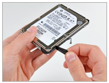
Remove the piece of tape covering the thermal sensor attached to the edge of the hard drive.
