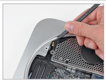
Use the tip of a spudger to carefully pry the antenna connector up off the AirPort/Bluetooth board.
