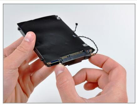
Remove the hard drive cable by pulling its connector straight away from the hard drive.
