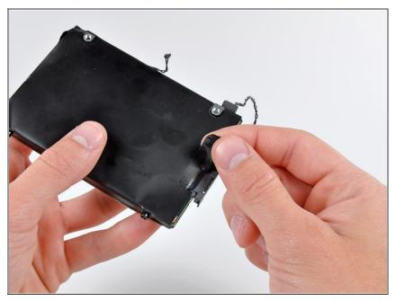
Remove the strip of tape covering the hard drive connector.
