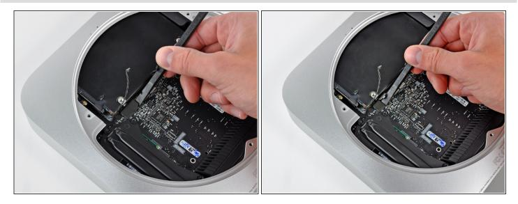
Use the flat end of a spudger to pry both the hard drive and optical drive connectors up out of their sockets on the logic board.
