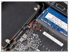
Simultaneously push the two plastic clips on the far left and right sides of the I/O board toward the middle of the I/O board and pull the I/O board slightly away from the outer case.
