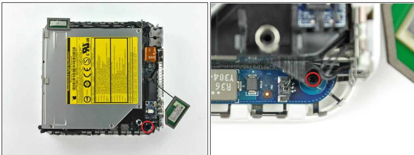
**i** In the next few steps, you will remove the four Phillips screws securing the internal frame to the bottom case. Included in each step is an overview picture showing the general location and a closeup showing the actual screw.
