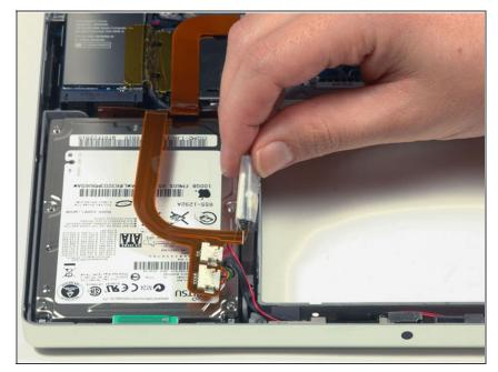
Slide the Bluetooth board out of its slot next to the hard drive. The Bluetooth board is still connected to the orange hard drive cable, so don't try to remove it entirely from the computer.
