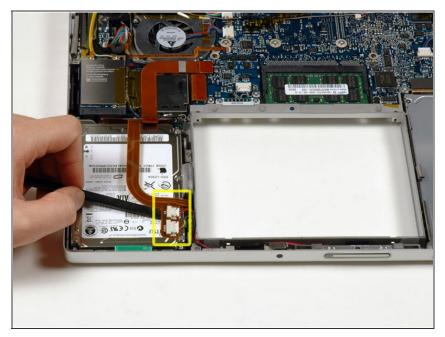
Use a spudger to carefully loosen the adhesive securing the sleep light and IR sensor connectors to the top of the hard drive.
