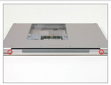
Rotate the computer 90 degrees and remove the two Phillips screws from the rear of the computer.
