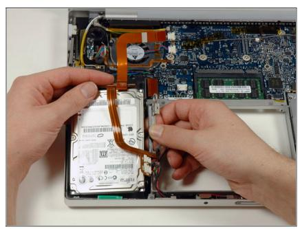
Lift the hard drive up with one hand and use your other hand to remove the retaining bracket from the side of the hard drive.
