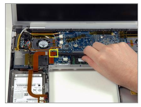
Disconnect the orange hard drive ribbon cable from the logic board.
