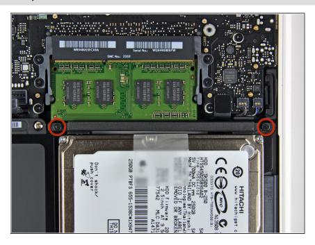
Remove two 11 mm Phillips screws securing the hard drive bracket to the upper case.
