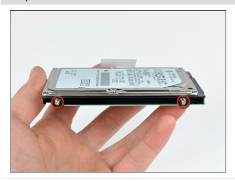
Remove the two T6 Torx screws from each side of the hard drive (four screws total).
