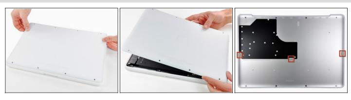
The lower case is constructed of rubber-coated aluminum. Do not excessively bend the aluminum during removal, as any permanent deformation will cause tolerance issues after reassembly.
