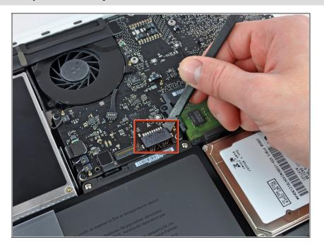
For precautionary purposes, we advise that you disconnect the battery connector from the logic board to avoid any electrical discharge. This step is **optional** and is not required.
