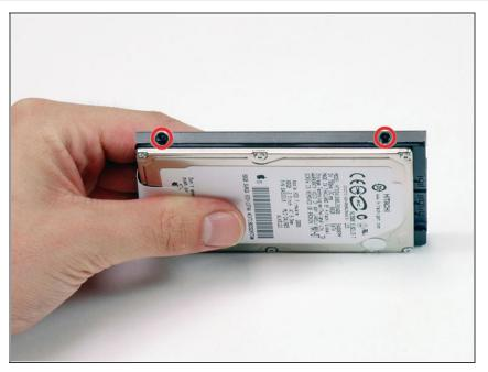
Rotate the hard drive and remove the two black T8 Torx screws on the other side of the drive.
