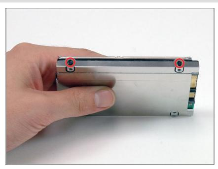
Remove the two black T8 Torx screws securing the silver bracket to the hard drive.
