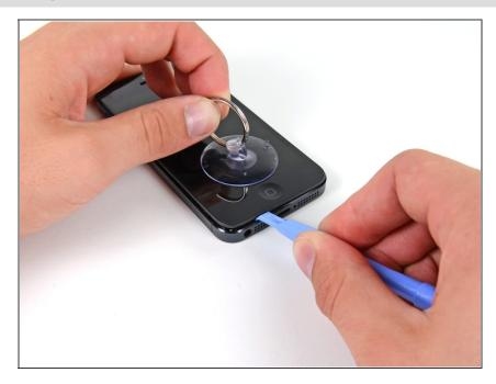
Make sure the suction cup is firmly attached to the front panel assembly.
