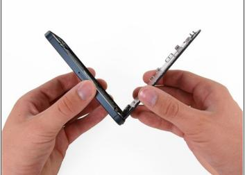
Do not try to completely remove the front panel assembly from the rear case, as there are several ribbon cables still attached at the top of the iPhone.
