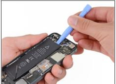
It may be possible to remove the battery simply by pulling on the plastic pull-tab. A slow continual pull seems to work best. If this is insufficient, proceed with the prying outlined in this step.
