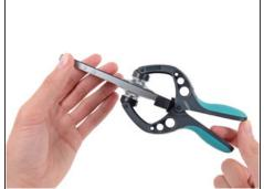
The next two steps demonstrate using the <u>iSclack</u>, a great tool for safely opening the iPhone 5 that we recommend for anyone doing more than one repair. If you aren't using the iSclack, skip to step 5.
