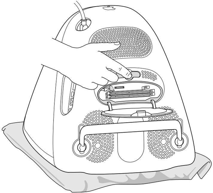
**Important:** To avoid electrostatic discharge, always ground yourself by touching the port access covers before you touch any parts or install any components inside the computer. To avoid static electricity building back up in your body, do not walk around the room until you have completed your installation and closed the computer.
