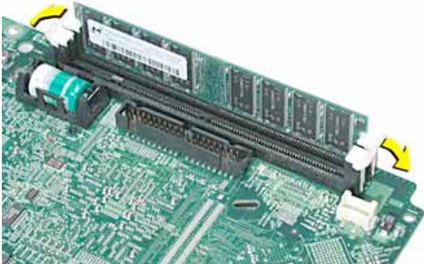
10. Insert the replacement memory into the open slot. The memory is designed to fit into the slot only one way. Be sure to align the notches on the module with the small notches inside the slot.
