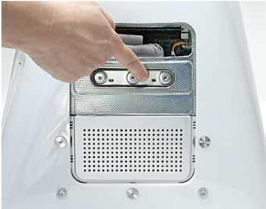
protect the computer from damage caused by electrostatic discharge. **Important:** To avoid electrostatic discharge, always ground yourself by touching metal before you touch any parts or install components inside the computer. To avoid generating static electricity, do not walk around the room until you have finished installing the memory and closed the computer.
