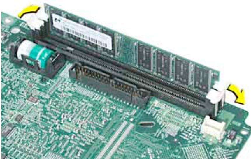
10. Push down on the memory until it snaps into place. The ejectors will automatically close.
