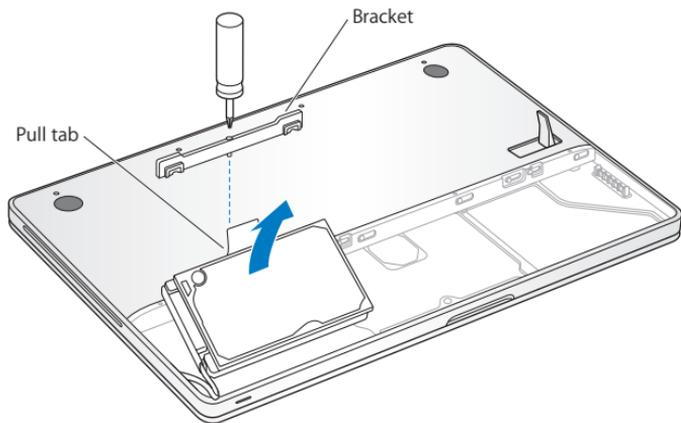
The bracket detaches from the drive. Put it aside in a safe place.
