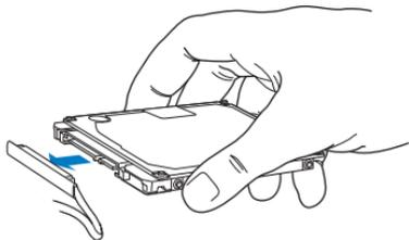
The connector is attached to a cable and remains in the hard disk drive bay.
