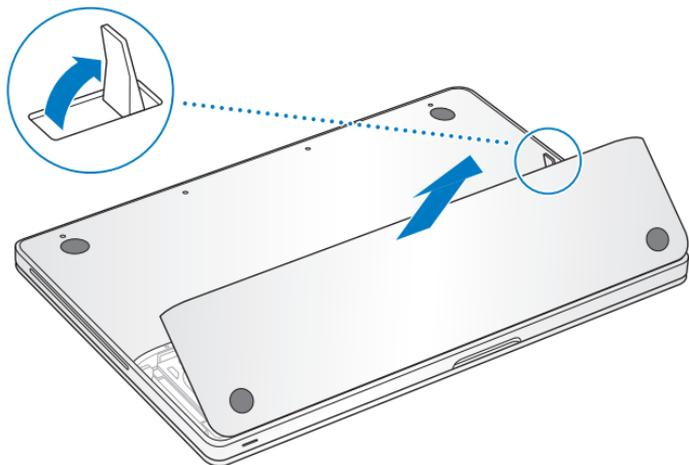
**Note:** The latch must be in its released, open position to remove and replace the battery and access door.
